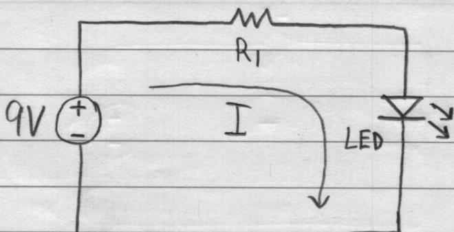
$V_F$  for LEDs depends on the size and color. For basic red, green, and yellow LEDs:  $V_F \approx 2.0V$  (see datasheet)
