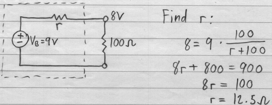
$r$  is not constant. Weaker battery has a higher  $r$ . Heavier load results in higher  $r$ .
