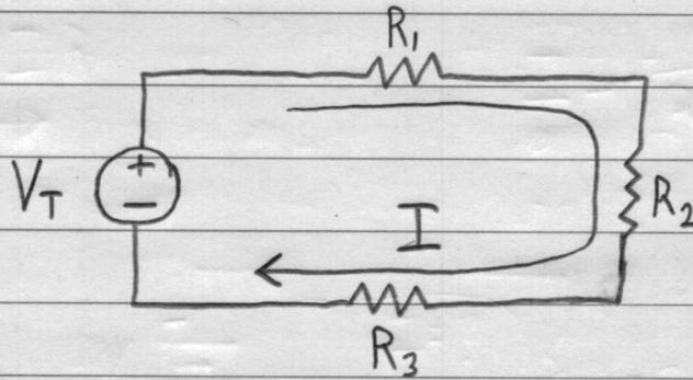
$$R_T = R_1 + R_2 + R_3$$
