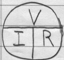
$$9V \begin{array}{c} + \\ \hline - \end{array} I = ? \quad R = 3\Omega \quad I = \frac{9V}{3\Omega} = 3A$$
